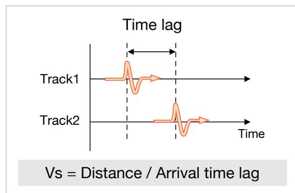
Fig. 4: Schematic showing the principles of SWM
