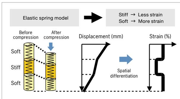
Fig. 2: Schematic showing the principles of RTE
