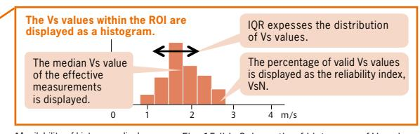
Fig. 15 (b): Schematic of histogram of Vs values
