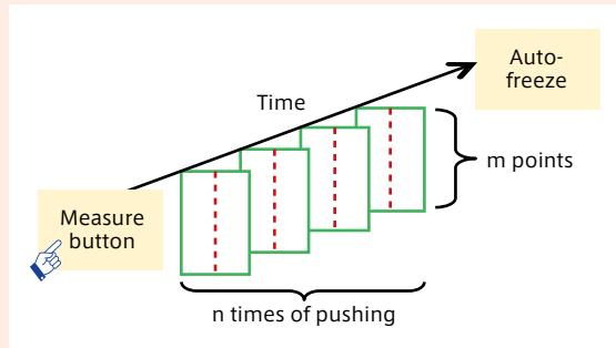
Fig. 16: Schematic of automatic multiple measurements
