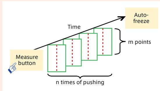
Fig. 16: Schematic of automatic multiple measurements
