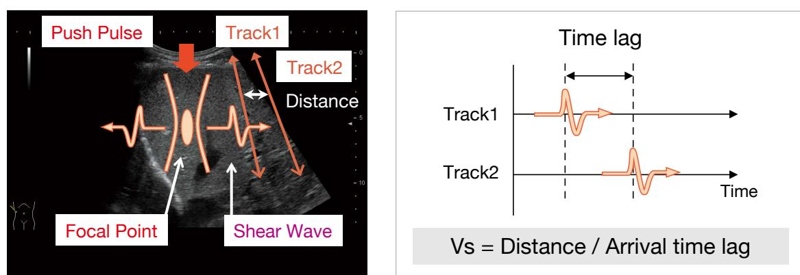
Fig. 4: Schematic showing the principles of SWM
